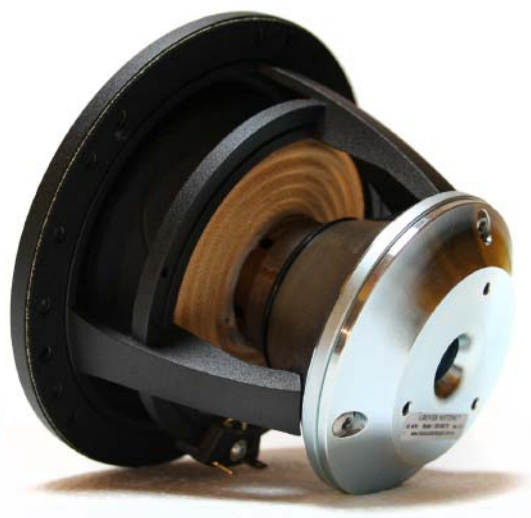
The unique Grover Notting driver showing the under-hung motor assembly.
